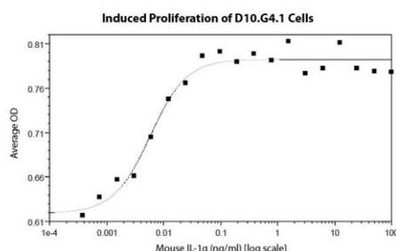
Induced proliferation of D10.G4.1 cells assay for Mouse IL-1  $\alpha$ . Cell proliferation was measured to calculate the ED50, which is as expected less than 10 pg/ml.
