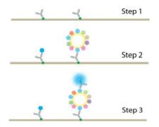
**Step 1:** Biotinylated antibody is bound to streptavidin coated assay plates. The kit provides a 96-well microplate with an 8-well strip format.
