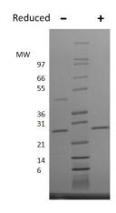
Non-reducing (-) and reducing (+) conditions in a 4 - 20% Tris-Glycine gel stained with Coomassie Blue. 1 µg of protein was loaded in each lane. Human CNTF has a predicted Mw of 22.9 kDa.
