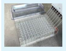
Incubate the plate for 1 hour at 37°C in an incubator
